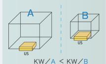
Watt density refers to the density of the workload that covers a specified range. Therefore, the higher the value, the more effective it is. The Beagle system divides the washing tank into upper and lower sections, which minimizes the volume. This makes the watt density higher than conventional systems, thereby making the washing much more effective.
